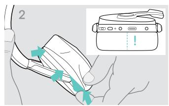
Insert the fixation band – stitched line facing to bottom – in the space on the ear cup.
